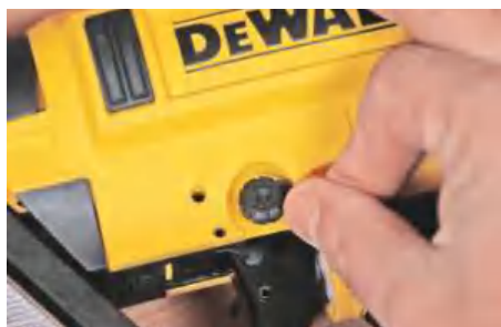
Bump and sequential firing is set with this dial
